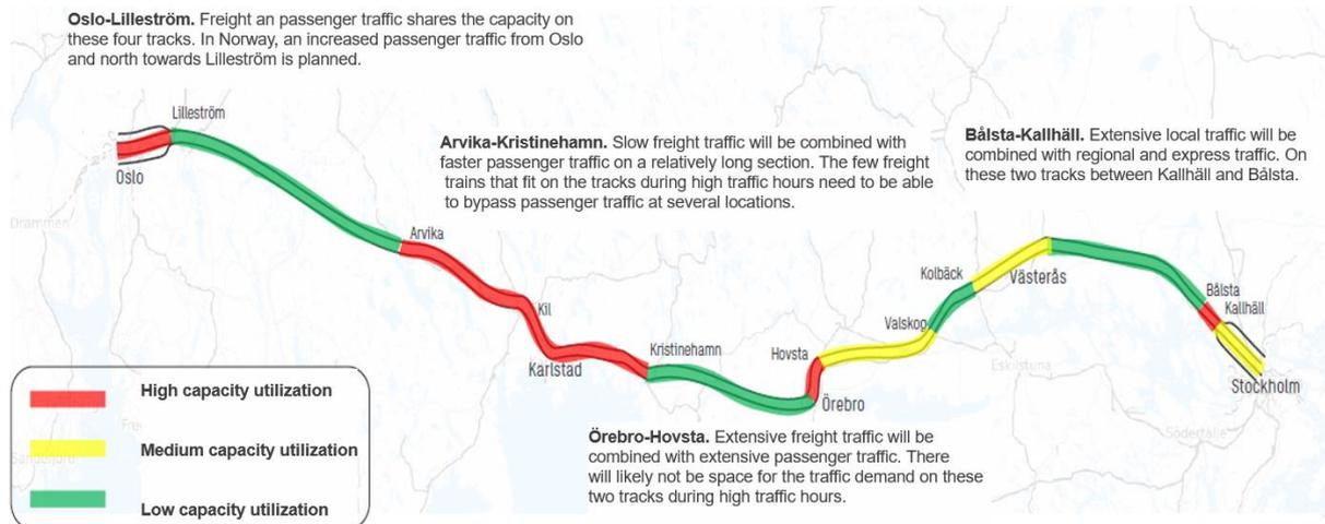
Figure 7 Capacity during high traffic hours, four traffic section, source: Sweco, 2018.
