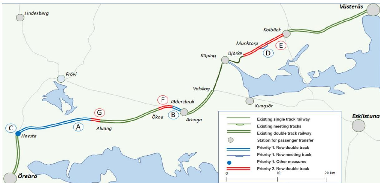
Figure 4 Measurement needs for the Örebro-Västerås section, for target year 2030, A-D correspond to priority 1 measures, E-G correspond to priority 2 measures, source: The Swedish Transport Administration, 2017b.
